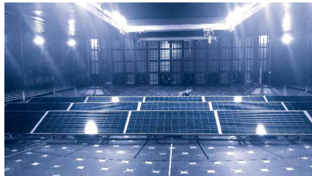
Full-scale solar array testing at the WindEEE Dome
